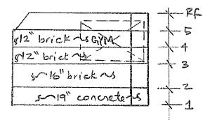
Elevation of zo's Partion showing wall thickness & material
